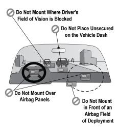
NOTE: The StreetPilot Bean Bag Dash Mount Accessory is designed to stabilize the unit during normal operation of a vehicle. It will not, however, secure the unit to the vehicle dash in the event of emergency braking or sharp turns. If you desire the added safety of a secure mount, use the StreetPilot Dash Mount Bracket and permanent adhesive supplied with the bracket.
